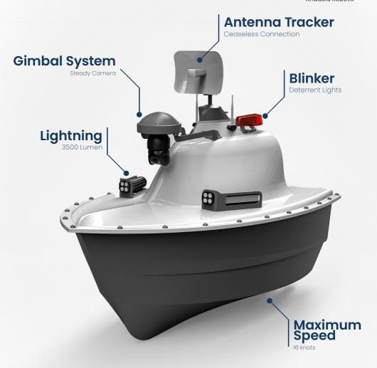
The developed unmanned patrol boat provides autonomous/manual operations in various areas and solves cost and security problems. Its high-torque engines perform even in harsh conditions with its composite or aluminum body options. The two communication systems cover a 40 km operational area; Its flexible structure makes customization possible. User interface provides fast and efficient control of surface operations.
